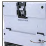
DIN35 rail mounting
