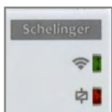
connection status indicator light
